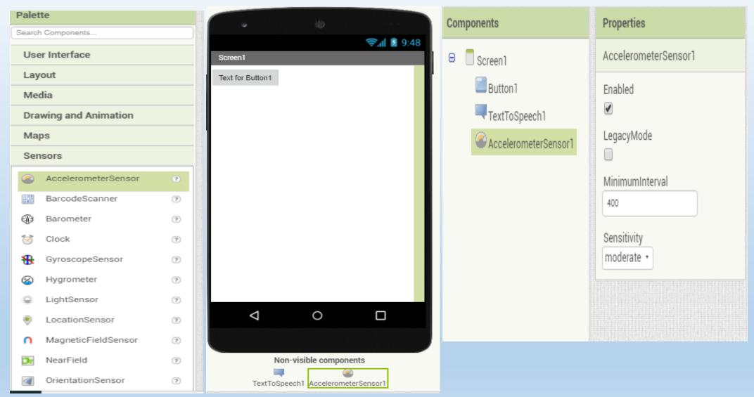
1- Click the AccelerometerSensor1 and Drag out the when accelerometerSensor1.Shaking do block.
